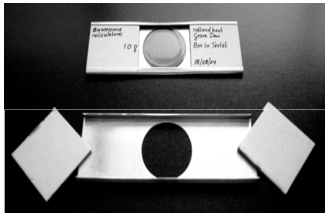
Fig: Prepared Cobb slide, and an aluminium holder with two cardboard pieces.
