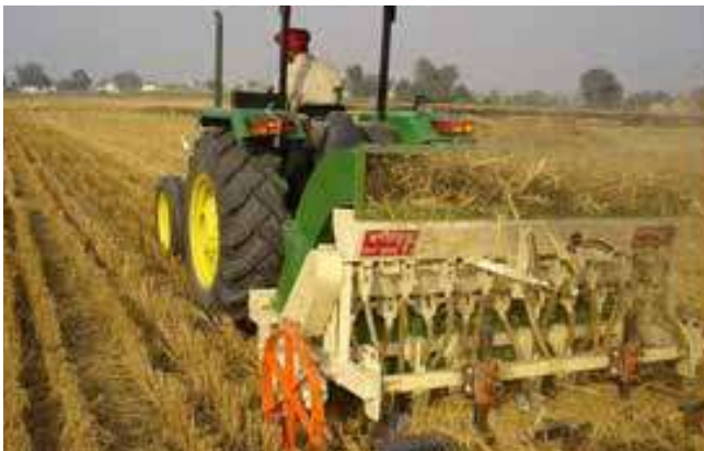
Jute sowing through Happy Seeder Technology in Wheat residues
